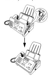
Reinsert the paper in the paper tray and push the paper release plate back down.
